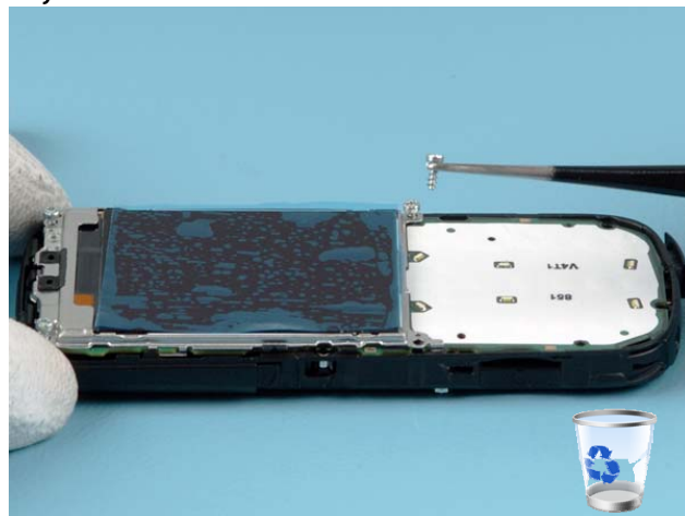
12b) Remove the screws with the tweezers. Do not use the screws again.
