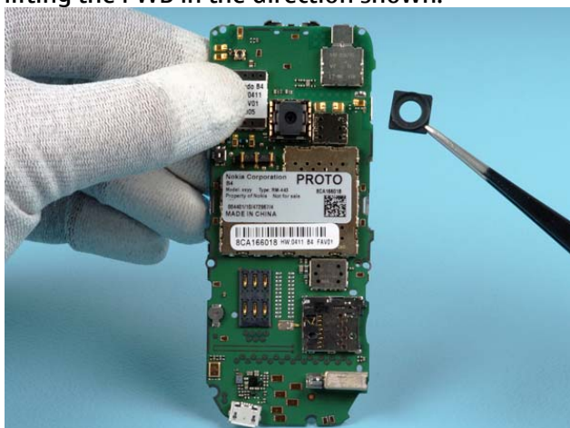
16b) Remove the CAMERA GASKET with the tweezers.
