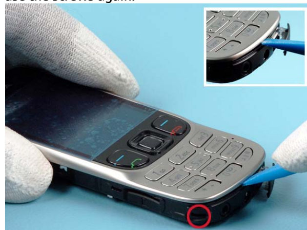
5) Release the bottom clip with the SS-93 tool.
