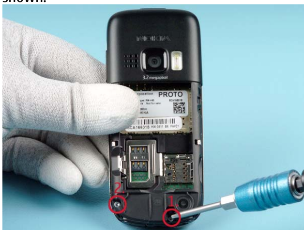
3a) Unscrew the two T6+ screws.
