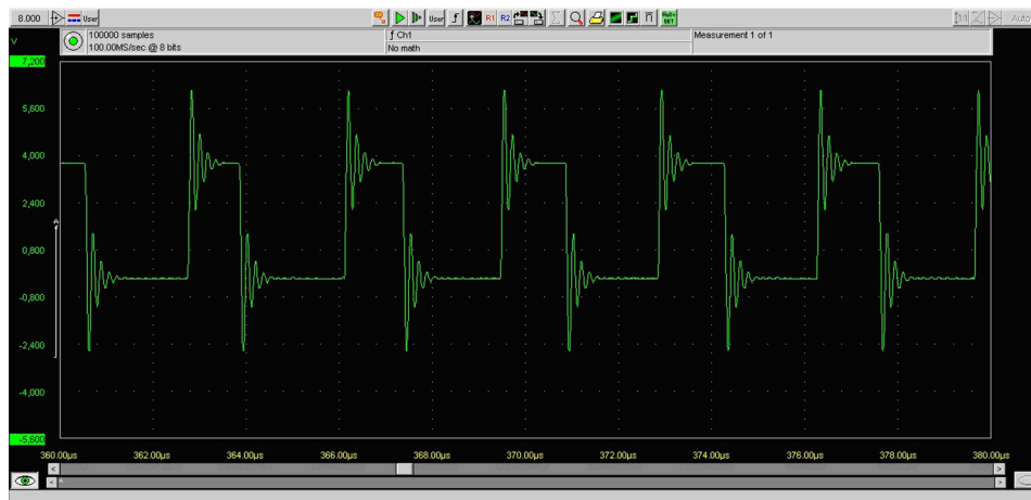
Figure 13 Single-ended output waveform of the Ext_in_IHF_out out loop measurement when speaker is connected (measured at speaker pads). No filter is used.
