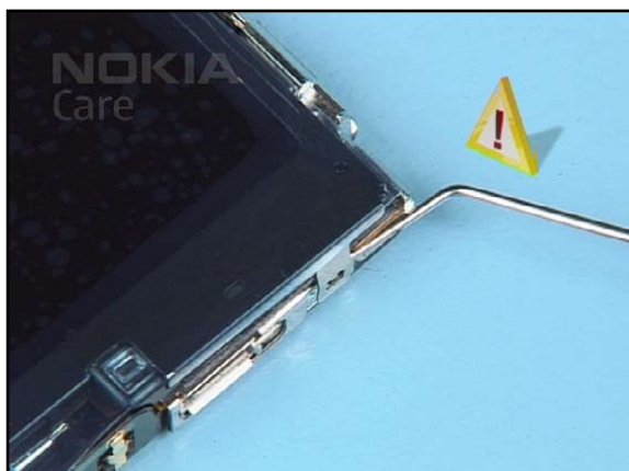
13. Open the clip on the top with the dental pick.
