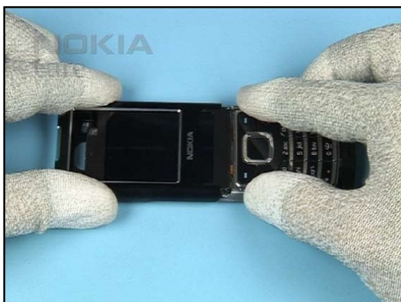
33. ...and carefully slide the A-Cover into its position.
