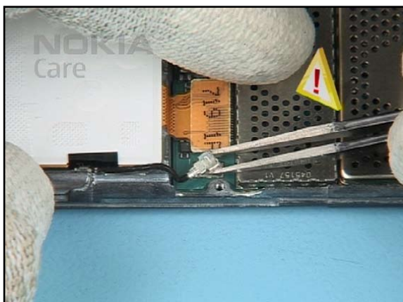
25. Carefully open the coax connector with tweezers.
