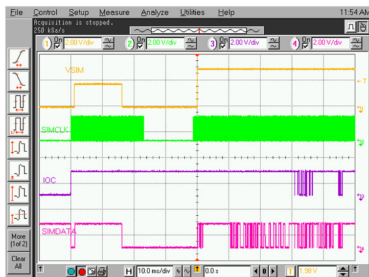
SIM power-on sequence between RAPU and EM ASIC.
