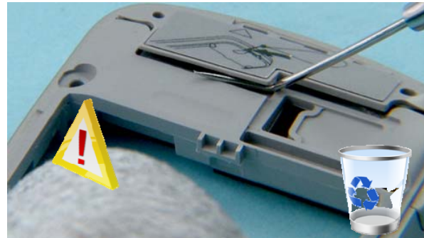
18) Carefully lift up the ANTENNA ASSY with the dental tool. The ANTENNA ASSY has always to be renewed.
