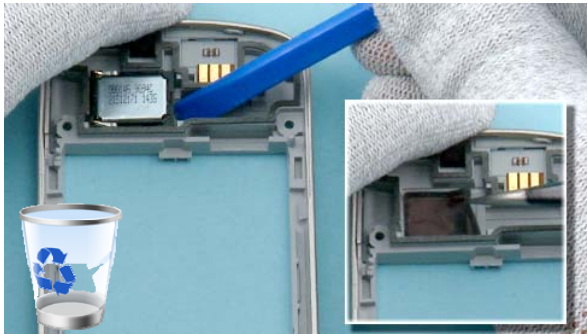
17) Use the SS-93 to lift up the IHF SPEAKER. Remove the IHF SPEAKER GASKET with the tweezers. The speaker, the speaker adhesive and the gasket cannot be reused.
