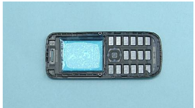
10) Protect also the other side of the A-COVER with protective film.
