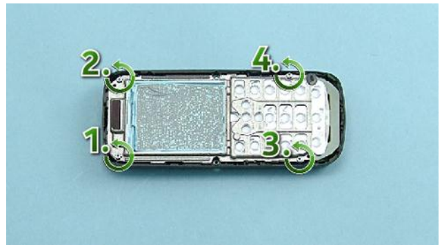
12) Unscrew the four TORX+ size 4 screws in the order shown.
