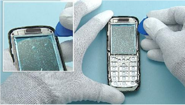
13) Open the clip with the SRT-6 to release the ENGINE BOARD.
