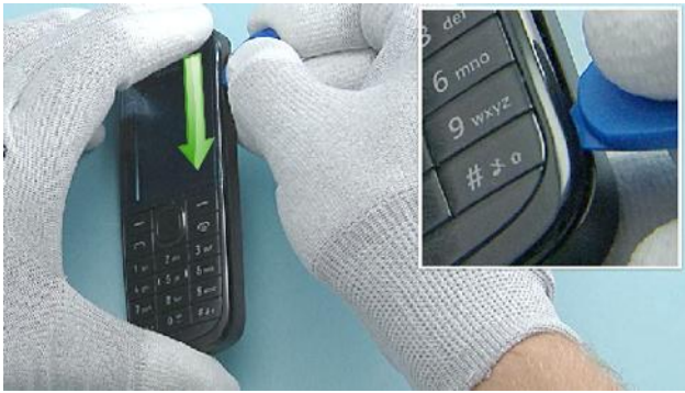
7) Release also the other side of the A-COVER with the SRT-6.
