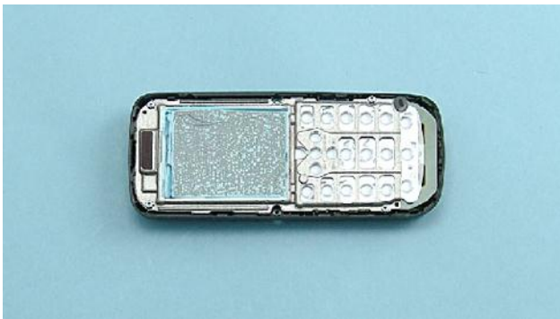
9) Protect the DISPLAY with protective film.
