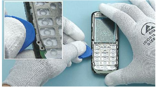
14) Open also the clip on the other side of the device with the SRT-6 to release the ENGINE BOARD.
